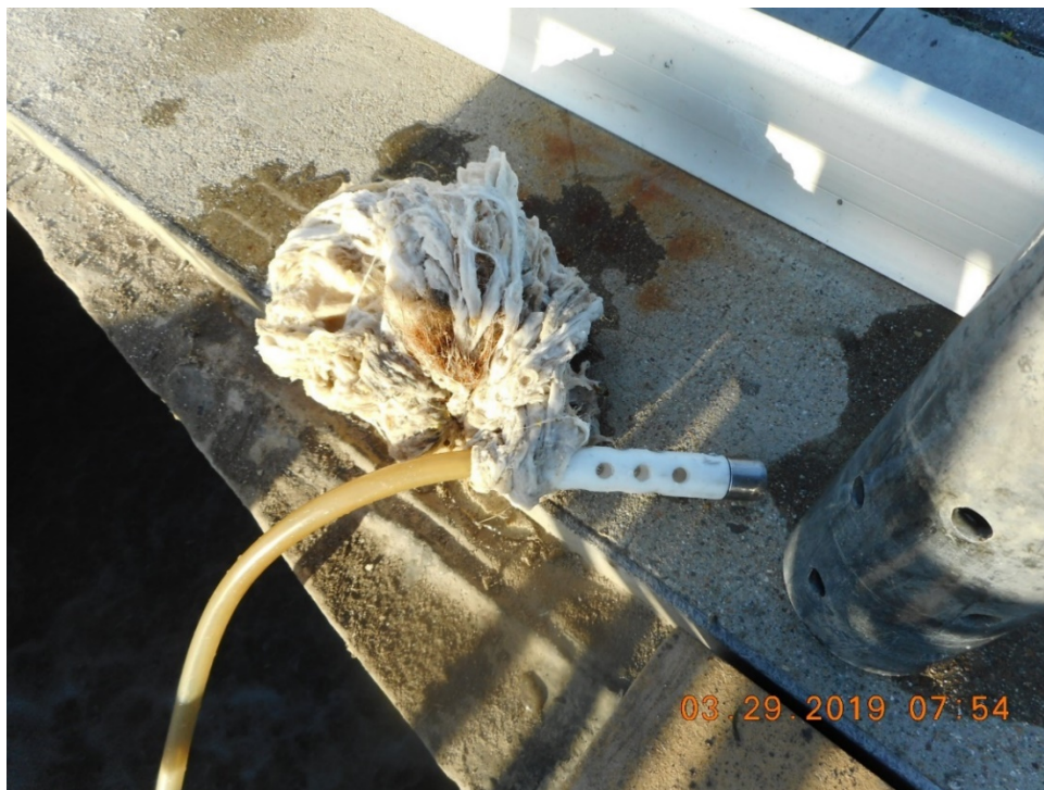
Figure 5-11 Rags Attached to Portable Sampler Intake Strainer on 3-29-19
